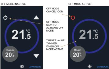
pressing the OFF icon. The system is designed so that the last command controls the current state. E.g. if the TRI has been overridden to OFF mode via the network, or a digital input transition, the user can cancel the OFF mode by pressing the OFF icon. Similarly a networked interface driven to OFF mode by the user can be overridden back to COMFORT mode using the network master.
