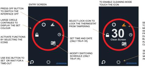
SELECT CLEANING ICON TO ENABLE CLEANING MODE. THE DISPLAY WILL COUNT DOWN FROM 30 SECONDS DURING WHICH ALL **BUTTONS ARE DISABLED** ALLOWING SCREEN CLEANING.
