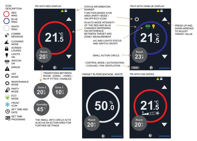
The TRI-1R room interface home screen has four touch sensitive areas that allow the system settings to be altered. All parameter values are available as Modbus/BACnet network variables. Fan speed and setpoint are available as 0-10Vdc outputs with TRI-3A.
